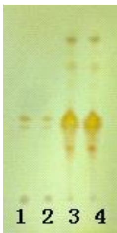
Figure S1. Thin-layer chromatographic analysis of non-alkaloids extract (NAE) and total dichloromethane extract by Dragendorff reagent. TLC was analysed on a Merck silica gel 60 F254 aluminum sheet with a mobile phase system including dichloromethane/methanol/formic acid (15:1:0.3) at ambient temperature. The same amount (1ml
