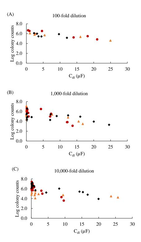
Fig. S6. The correlation between the log colony counts of biofilm (log CFU swab<sup>-1</sup>) and  $C_{dl}$  of three replicates ( $\spadesuit$ ,  $\bullet$ , and  $\blacktriangle$ ) of the 100-fold (A), 1,000-fold (B), or 10,000-fold (C) dilution experiment (based on the biofilm model).
