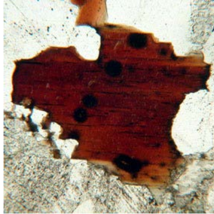
A biotite crystal shows brown pleochroic behaviour as the stage is rotated.
