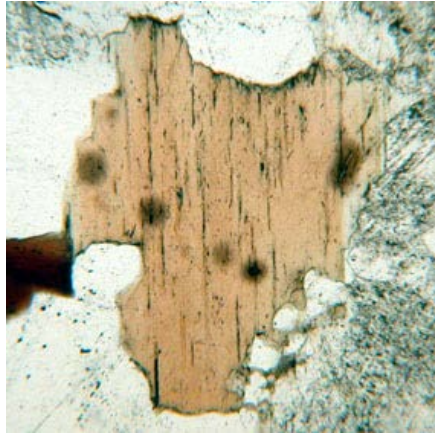
A biotite crystal shows brown pleochroic behaviour as the stage is rotated.
