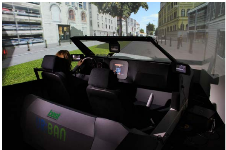
2 3 Fig. A1. BAST driving simulator. The driver's cabin, the touch display with the secondary 4 task, and the representation of traffic and environment can be seen.
