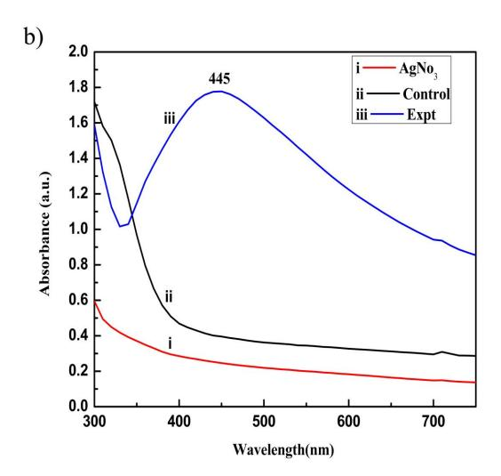
**Supplementary Figure 1.** (a) Schematic diagram of Pb-AgNPs synthesis exposed to sunlight; (b) UV–Vis spectra of (i) AgNO<sub>3</sub>, (ii) Control (*P. betle* leaf extract) and (iii) Experimental (Pb-AgNPs).
