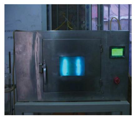
Figure 10. Experimental instrument for the MW/UV catalytic oxidation of the wastewater mixture. Four microwave electrodeless lamps, which are fixed in the middle of the microwave chamber, produce UV light under microwave radiation. In the upper right corner of the instrument, there is an auto digital display power-controlling unit, which is used to automatically control power, time and temperature of the reaction.
