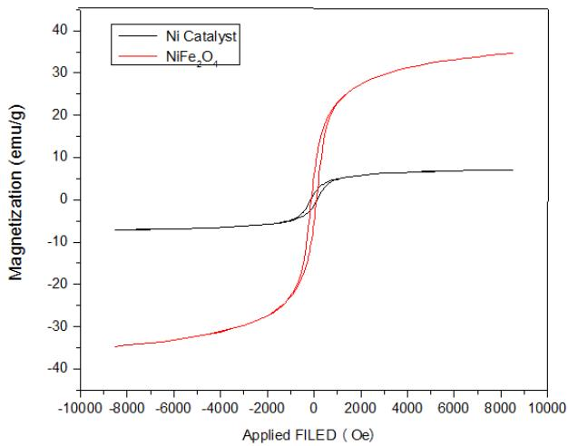
Fig. S2. The vibrating sample magnetometer curve of  $\text{NiFe}_2\text{O}_4$  nanoparticles and  $\text{NiFe}_2\text{O}_4@\text{TASDA-Pd}(0)$ .
