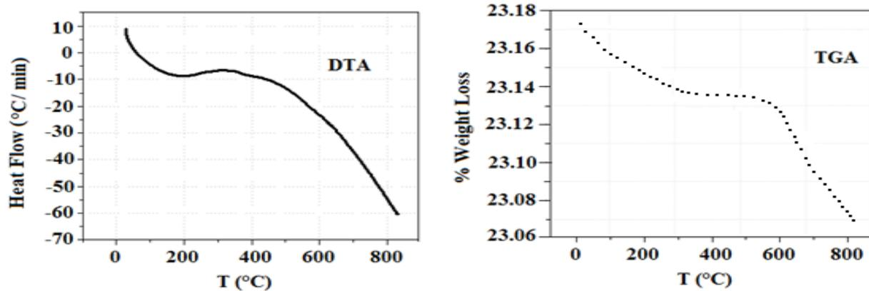
**Fig S3.** Thermogravimetric analysis (TGA) and differential thermal analysis (DTA) of CuO NPs.
