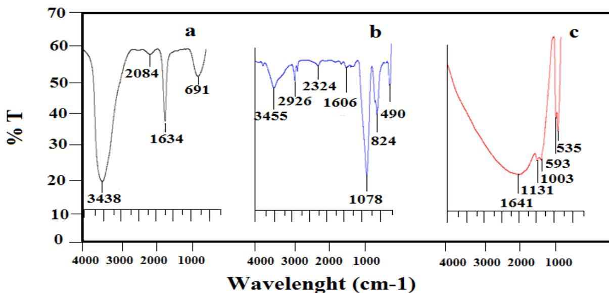
**Fig. S2.** FTIR of green synthesized CuO NPs. (a) Leave Extract (b) Reaction Mixture (c) CuO NPs
