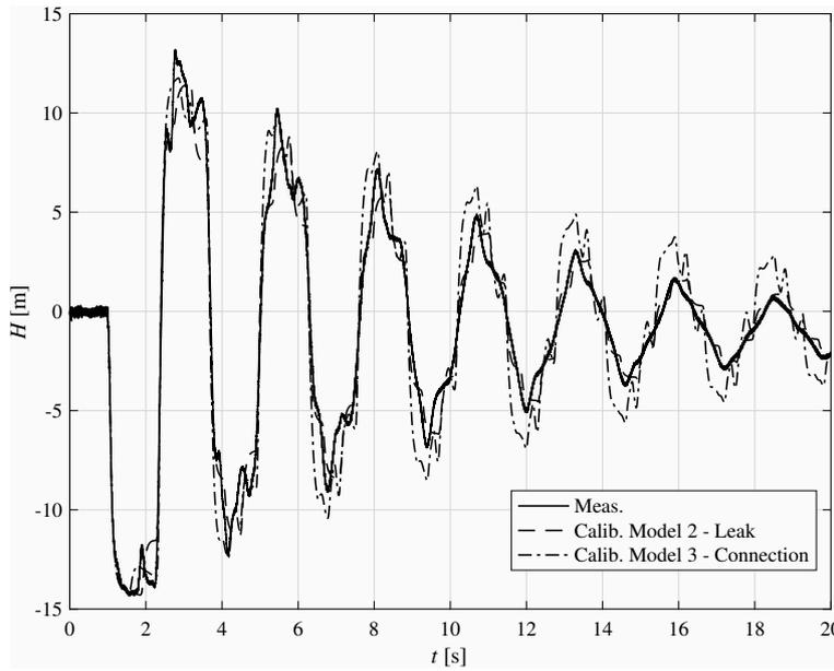
Figure B2.: Comparison of  $H$  measured at the pressure transducer (Meas.) with results of the calibration of the models with a leak (dashed line, Model 2) or an illegal connection (dash dotted line, Model 3) in the system, corresponding to the minima of  $\sigma_2^2$ .
