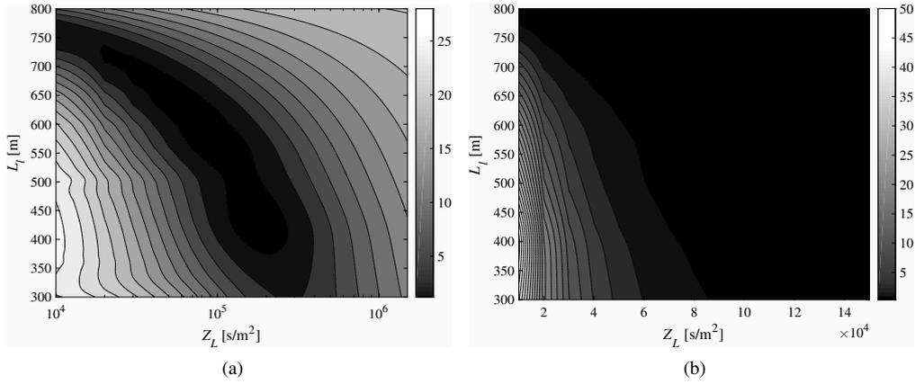
Figure B1.: Variation of (a)  $\sigma_1^2$  and (b)  $\sigma_2^2$  with the leak location,  $L_1$ , and impedance,  $Z_L$ , in Model 2 of Fig. 3.
