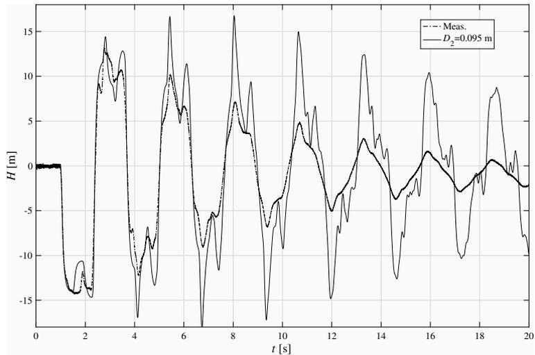
Figure B5.: Comparison of  $H$  measured at the pressure transducer (Meas.) and obtained by the calibration of Model 4, with a trunk of diameter  $D_2$  (dash dotted line), corresponding to the minima of  $\sigma_2^2$ .
