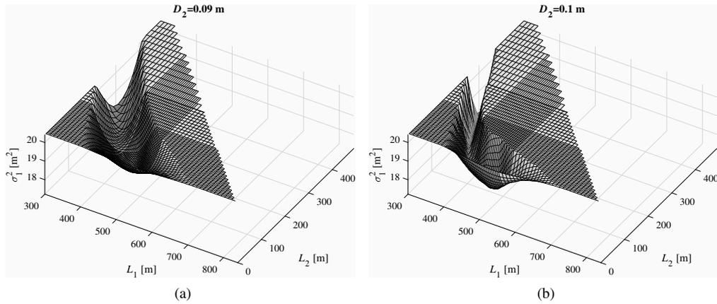
Figure B4.: Variation of  $\sigma_2^2$  with the pipe with a different diameter,  $D_2$ , of length,  $L_2$  and at a distance  $L_1$  from the upstream node (Model 4 of Fig. 3).
