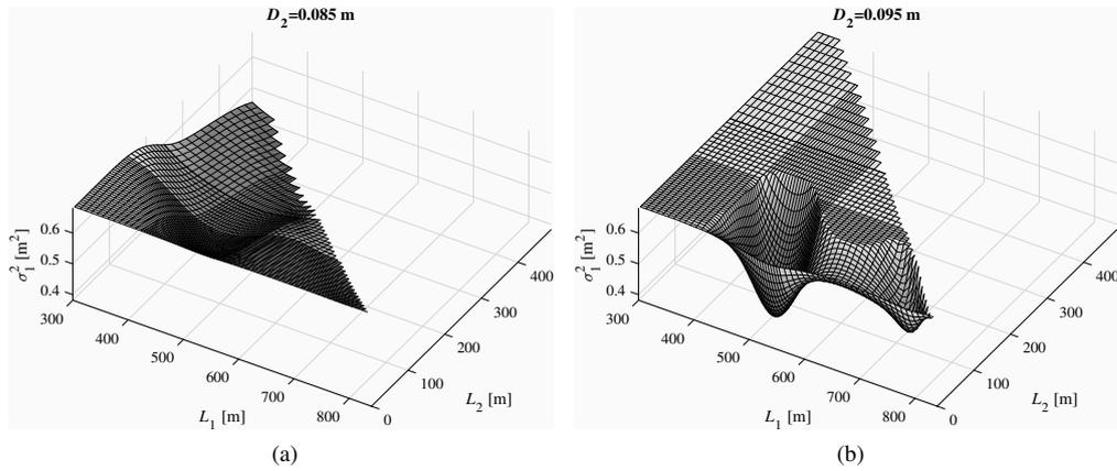
Figure B3.: Variation of  $\sigma_1^2$  for a pipe with a different diameter,  $D_2$ , of length  $L_2$  and at a distance  $L_1$  from the upstream node (Model 4 of Fig. 3).
