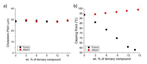
Figure S6. (a) Pitch and (b) clearing point of a cholesteric LC containing various amounts of pyrene or RM257. Cholesteric LC contained 0.3 wt. % of S-811. Characterization of the pitch was performed at room temperature.
