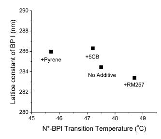
Figure S5. Lattice constant of BP I at the N\*-BP I transition temperature of BPs 1 wt. % of containing various additives.
