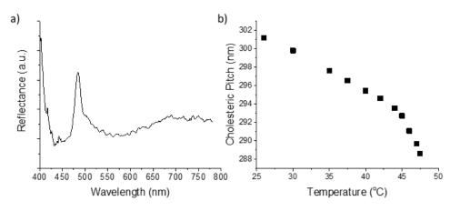
Figure S2. (a) Reflection spectrum obtained from a BP-forming cholesteric LC (containing 32.5 wt.% of S-811) at room temperature. Peak at 492 nm corresponds to Bragg reflection due to helical distortion of the LC director. (b) Pitch of helical director in the cholesteric LC as function of temperature.
