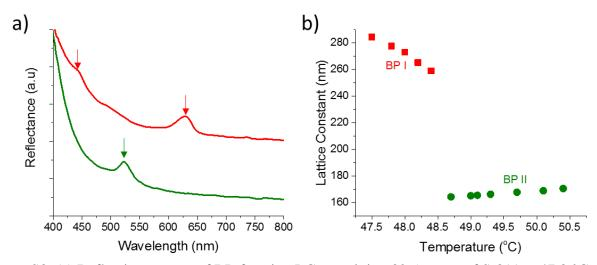
Figure S3. (a) Reflection spectra of BP-forming LC containing 32.5 wt. % of S-811 at 47.8 °C (red trace) and 48.7 °C (green trace). (b) Lattice constants of BP I (red squares) and BP II (green circles) as a function of temperature.
