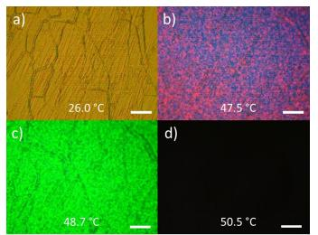
Figure S1. Images of a BP-forming LC containing 32.5 wt. % of S-811 at different temperatures: (a) 26.0 °C (cholesteric phase); (b) 47.5 °C (BP I phase); (c) 48.7 °C (BP II phase); and (c) 50.5 °C (isotropic phase). Image (a) was obtained with a crossed-polarized light microscopy using transmitted-light illumination. Images (b)-(d) were obtained using reflected-light illumination. Scale bar corresponds to 100  $\mu$ m.
