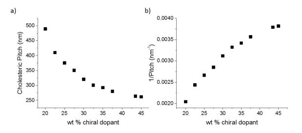
Figure S4. (a) Pitch of cholesteric LCs as a function of the weight percent of the chiral dopant (S-811). Data obtained at room temperature (26  $^{\circ}$ C). (b) Plot of inverse of the pitch against the concentration of chiral dopant in the LC.
