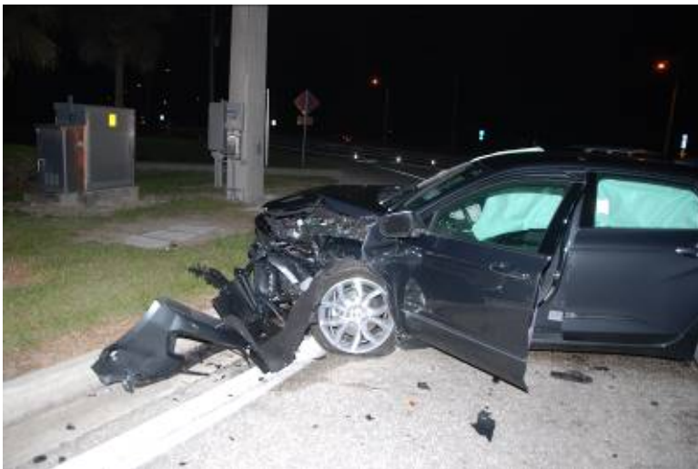
Figure A3. A head-on collision between this 2015 Chevrolet Impala and a passenger car resulted in a 44 km/h longitudinal delta V (from EDR) for the Impala. Both rear-seat occupants, an 84-year-old obese male in the left rear and a 79-year-old obese female in the right rear, were fatally injured with chest and spine injuries.
