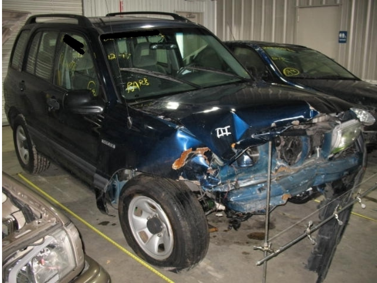
Figure A2. A head-on collision between this 2002 Suzuki Vitara and a passenger car resulted in an estimated 19 km/h delta V (from crash reconstruction) for the Vitara. A 64-year-old female in the left rear seat was fatally injured with AIS 3+ chest and head injuries.
