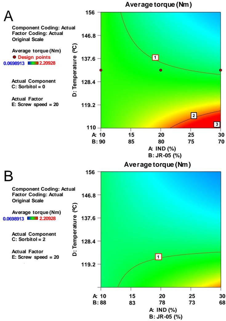
**Supp. Figure 6.** Influence of IND/JR-05 and temperature on average torque (Nm) in screw speed at 20 rpm: (A) Sorbitol 0%: (B) Sorbitol 2% in Mix-process plot.
