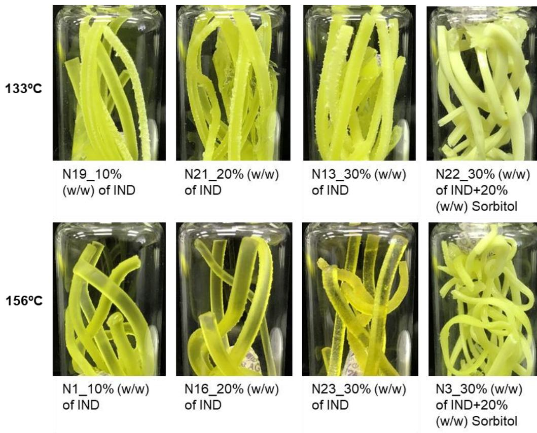
**Supp. Figure 2.** Examples for the physical appearance of melt extrudate consisted of IND (10% to 30%) and JR-05 with or without Sorbitol (20%) processed at 133°C and 156°C.
