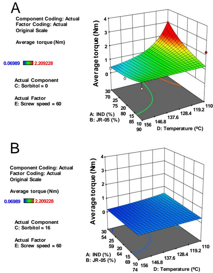
**Supp. Figure 1.** Influence of IND/JR-05 and temperature on average torque (Nm) in screw speed at 60 rpm: (A) Sorbitol 0 %: (B) Sorbitol 16% in three-dimensional Mix-process plots.
