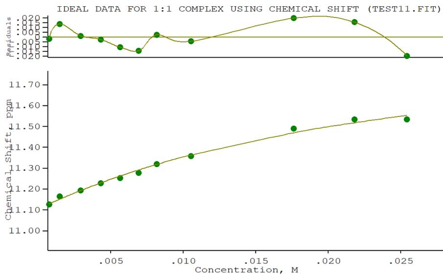
**Figure S42.** Fitted binding isotherm obtained for the titration of a 0.005 M solution of compound **L8** with a 0.075 M solution of TBACl ( $\text{DMSO-}d_6$ ). The graph shows the change in chemical shift of the signal of the NH protons of the molecule, fitted to a 1:1 ( $\text{L}:\text{Cl}^-$ ) binding model.
