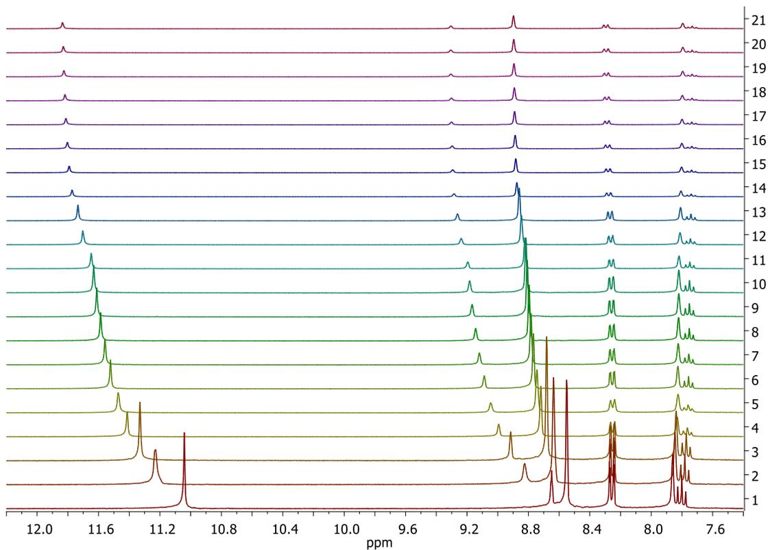
**Figure S33.** Excerpt of the  $^1\text{H}$  NMR spectra (300 MHz,  $\text{DMSO-}d_6$ ) obtained upon addition of different aliquots of a 0.1 M solution of TBACl to a 0.01 M solution of **L4**.
