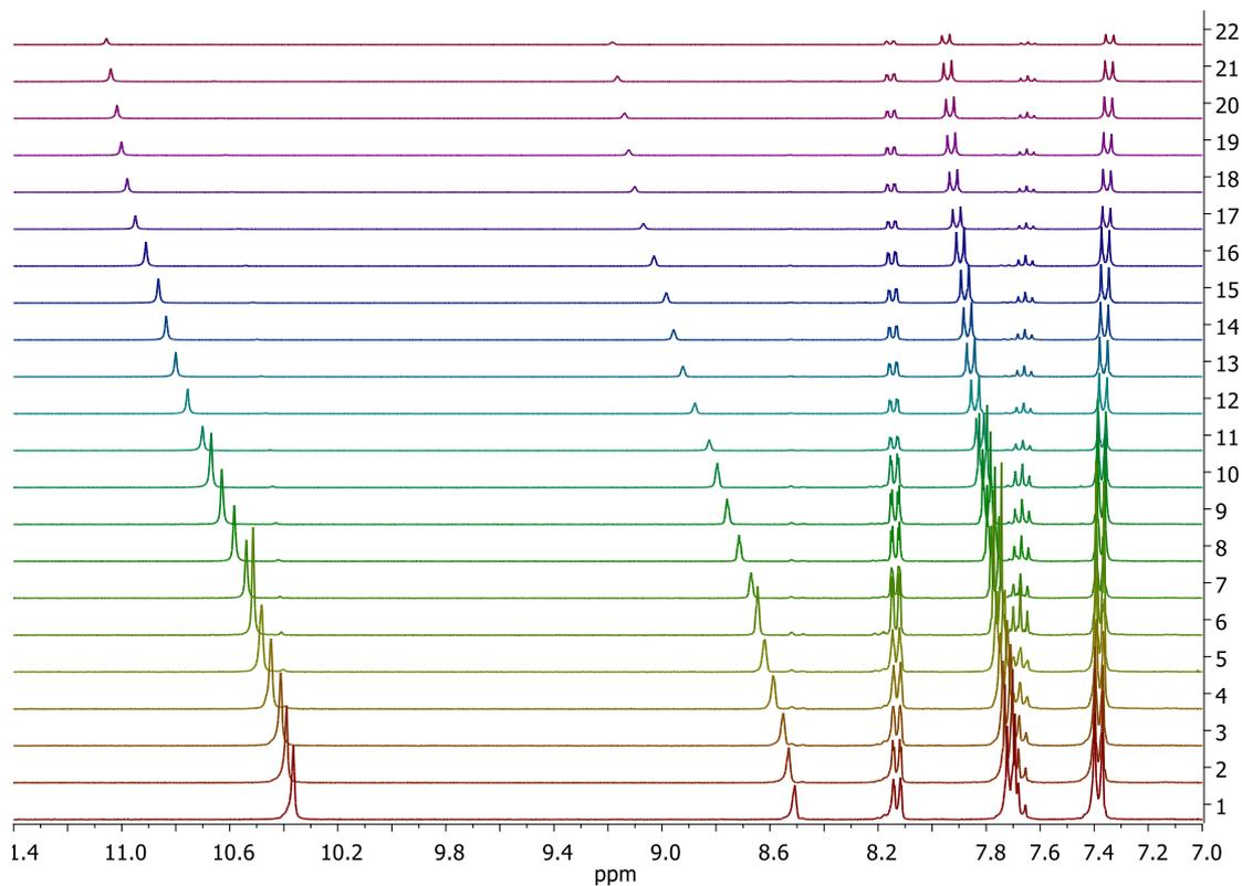
**Figure S29.** Excerpt of the  $^1\text{H}$  NMR spectra (300 MHz,  $\text{DMSO-}d_6$ ) obtained upon addition of different aliquots of a 0.1 M solution of TBACl to a 0.01 M solution of **L2**.
