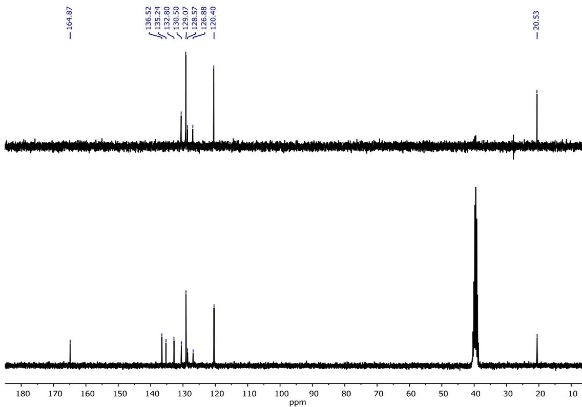
Figure S3.  $^{13}\text{C}$  and DEPT NMR spectra (75 MHz,  $\text{DMSO-}d_6$ ) for compound L1.
