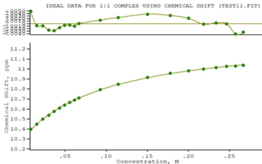
**Figure S28.** Fitted binding isotherm obtained for the titration of a 0.01 M solution of compound **L1** with a 0.1 M solution of TBACl ( $\text{DMSO-}d_6$ ). The graph shows the change in chemical shift of the signal of the NH protons of the molecule, fitted to a 1:1 ( $\text{L}:\text{Cl}^-$ ) binding model.
