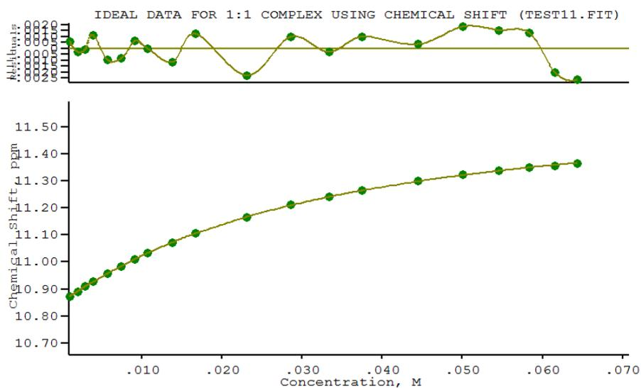
**Figure S38.** Fitted binding isotherm obtained for the titration of a 0.01 M solution of compound **L6** with a 0.1 M solution of TBACl ( $\text{DMSO-}d_6$ ). The graph shows the change in chemical shift of the signal of the NH protons of the molecule, fitted to a 1:1 ( $\text{L}:\text{Cl}^-$ ) binding model.
