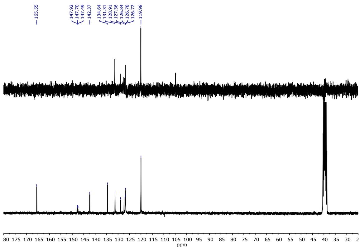
Figure S18.  $^{13}\text{C}$  and DEPT NMR spectra (75 MHz,  $\text{DMSO-}d_6$ ) for compound L6.
