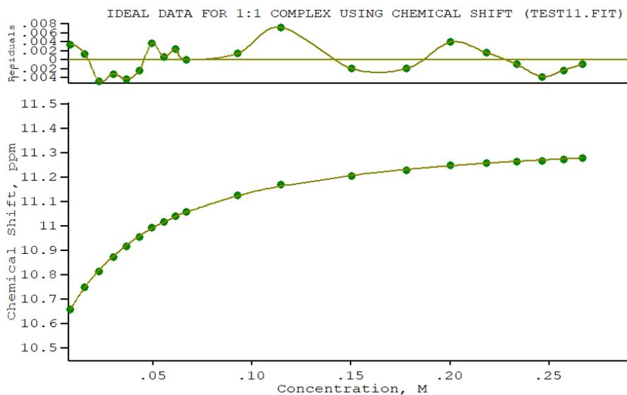
**Figure S32.** Fitted binding isotherm obtained for the titration of a 0.01 M solution of compound **L3** with a 0.1 M solution of TBACl ( $\text{DMSO-}d_6$ ). The graph shows the change in chemical shift of the signal of the NH protons of the molecule, fitted to a 1:1 ( $\text{L}:\text{Cl}^-$ ) binding model.
