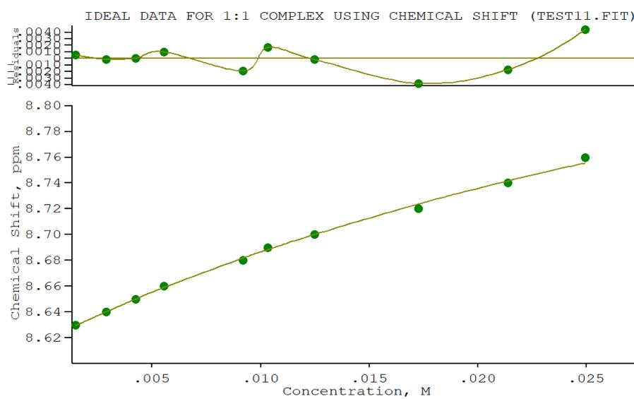
**Figure S40.** Fitted binding isotherm obtained for the titration of a 0.005 M solution of compound **L7** with a 0.075 M solution of TBACl ( $\text{DMSO-}d_6$ ). The graph shows the change in chemical shift of the signal of the NH protons of the molecule, fitted to a 1:1 ( $\text{L}:\text{Cl}^-$ ) binding model.
