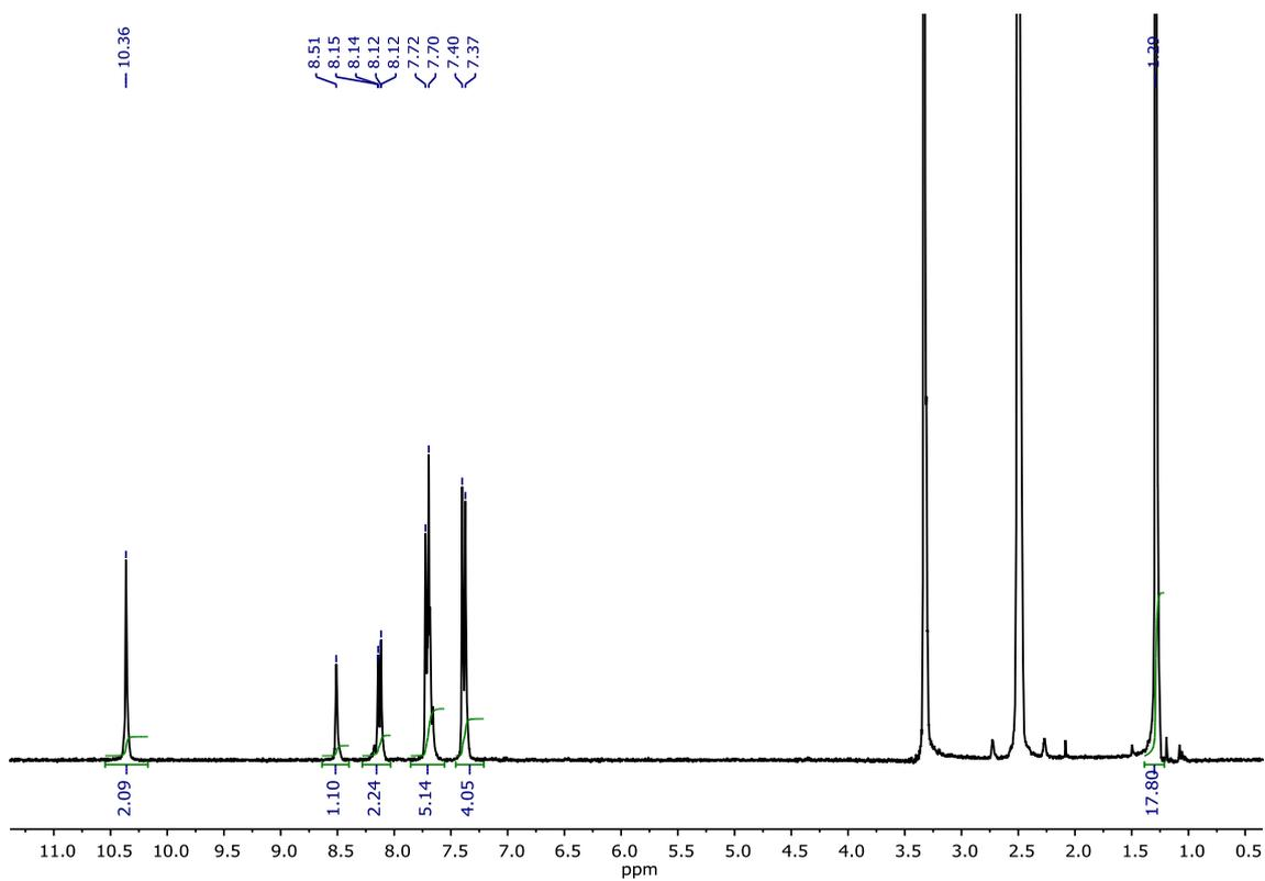
Figure S5.  $^1\text{H}$  NMR spectrum (300 MHz,  $\text{DMSO-}d_6$ ) for compound L2.
