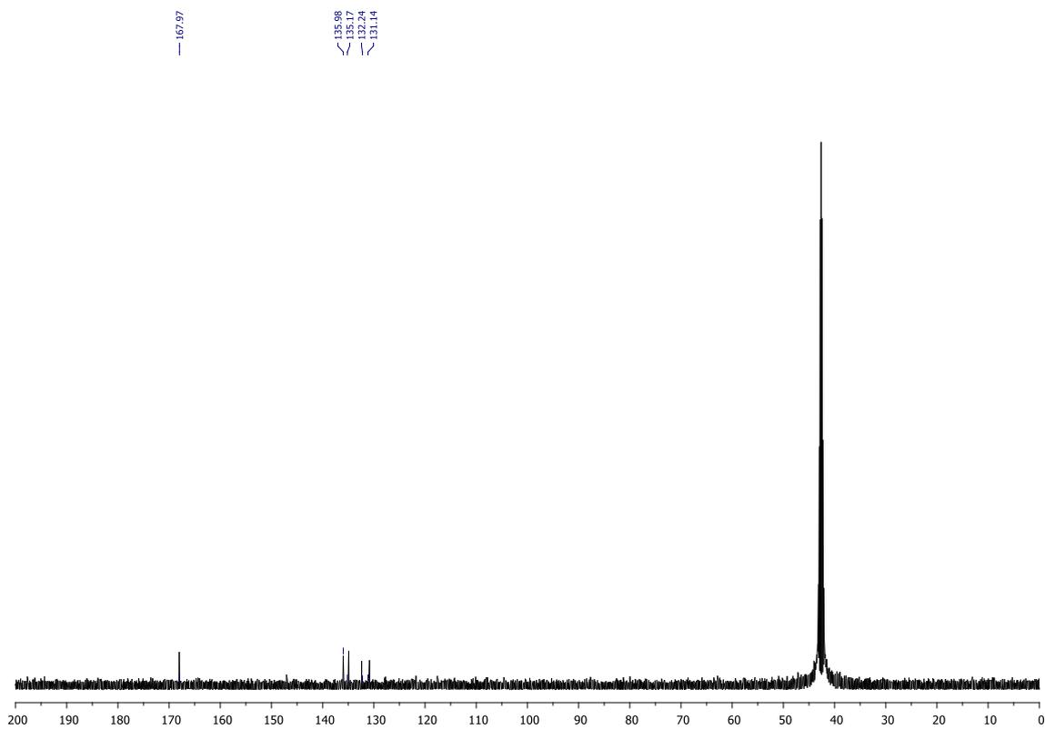
Figure S21.  $^{13}\text{C}$  NMR spectrum (75 MHz,  $\text{DMSO-}d_6$ ) for compound L7.
