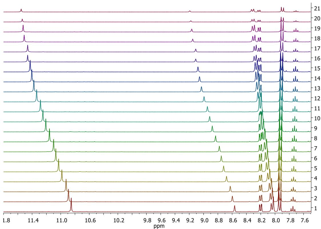
**Figure S37.** Excerpt of the  $^1\text{H}$  NMR spectra (300 MHz,  $\text{DMSO-}d_6$ ) obtained upon addition of different aliquots of a 0.1 M solution of TBACl to a 0.01 M solution of **L6**.
