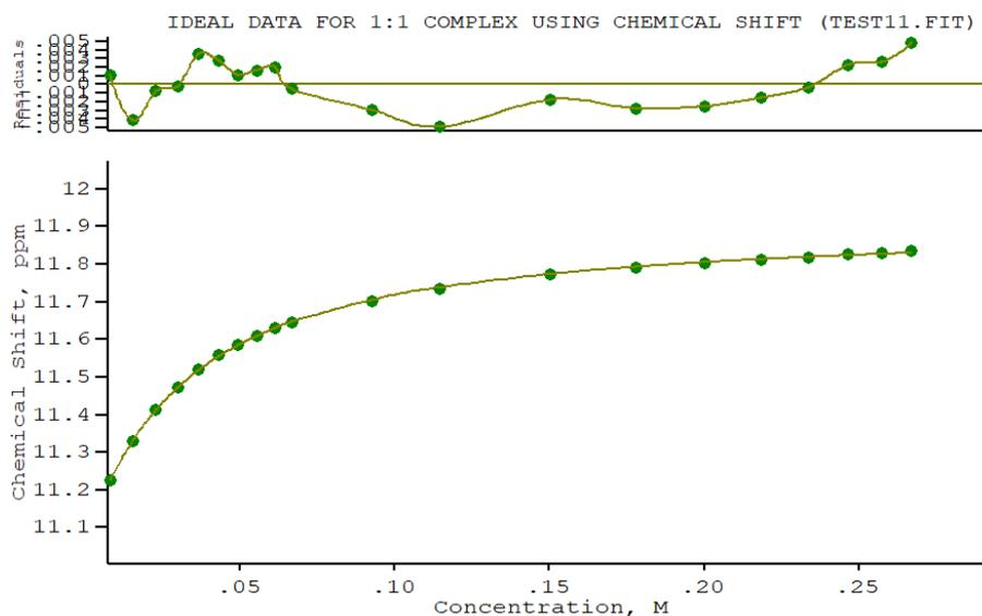
**Figure S34.** Fitted binding isotherm obtained for the titration of a 0.01 M solution of compound **L4** with a 0.1 M solution of TBACl ( $\text{DMSO-}d_6$ ). The graph shows the change in chemical shift of the signal of the NH protons of the molecule, fitted to a 1:1 ( $\text{L}:\text{Cl}^-$ ) binding model.
