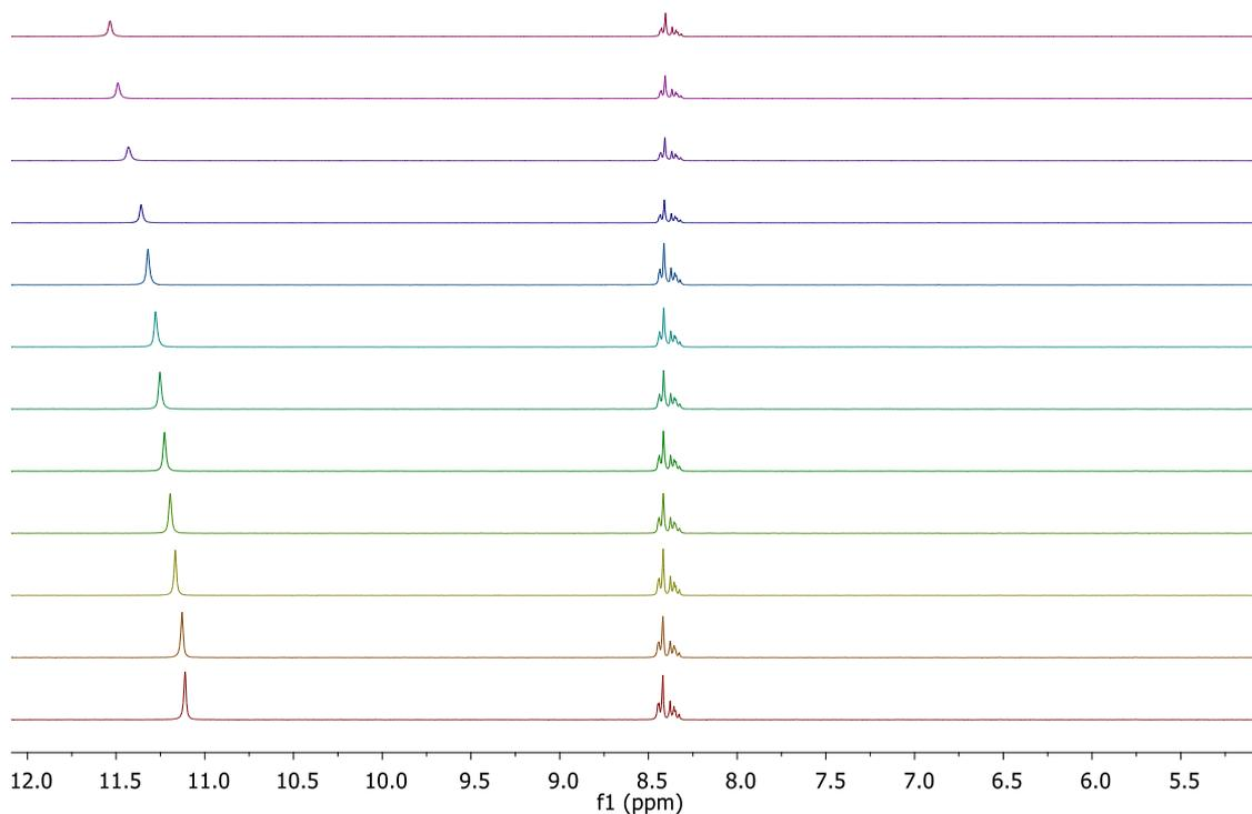
**Figure S41.** Excerpt of the  $^1\text{H}$  NMR spectra (300 MHz,  $\text{DMSO-}d_6$ ) obtained upon addition of different aliquots of a 0.075 M solution of TBACl to a 0.005 M solution of **L8**.
