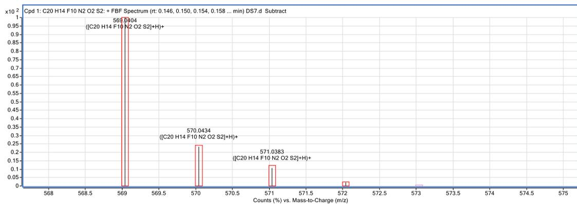
**Figure S19.** HR-MS (+ESI) spectrum for compound L6.
