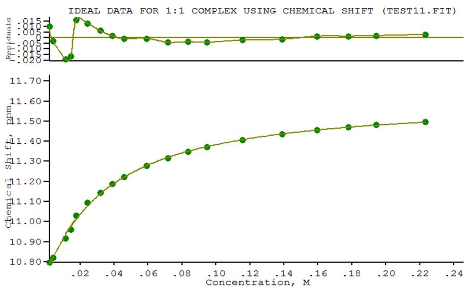
**Figure S36.** Fitted binding isotherm obtained for the titration of a 0.01 M solution of compound **L5** with a 0.1 M solution of TBACl ( $\text{DMSO-}d_6$ ). The graph shows the change in chemical shift of the signal of the NH protons of the molecule, fitted to a 1:1 ( $\text{L}:\text{Cl}^-$ ) binding model.
