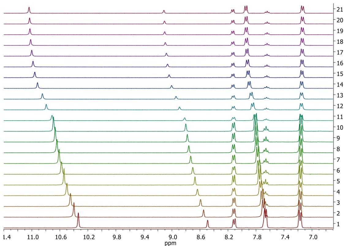
**Figure S27.** Excerpt of the  $^1\text{H}$  NMR spectra (300 MHz,  $\text{DMSO-}d_6$ ) obtained upon addition of different aliquots of a 0.1 M solution of TBACl to a 0.01 M solution of **L1**.
