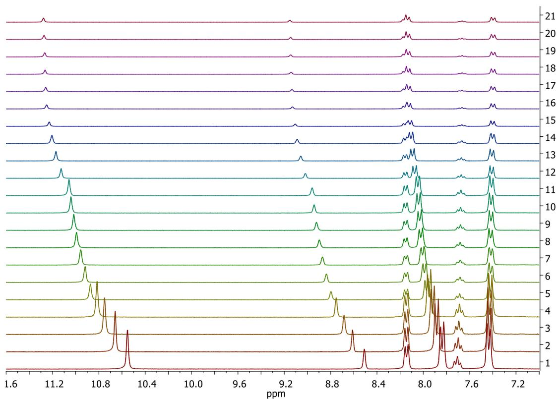
**Figure S31.** Excerpt of the  $^1\text{H}$  NMR spectra (300 MHz,  $\text{DMSO-}d_6$ ) obtained upon addition of different aliquots of a 0.1 M solution of TBACl to a 0.01 M solution of **L3**.
