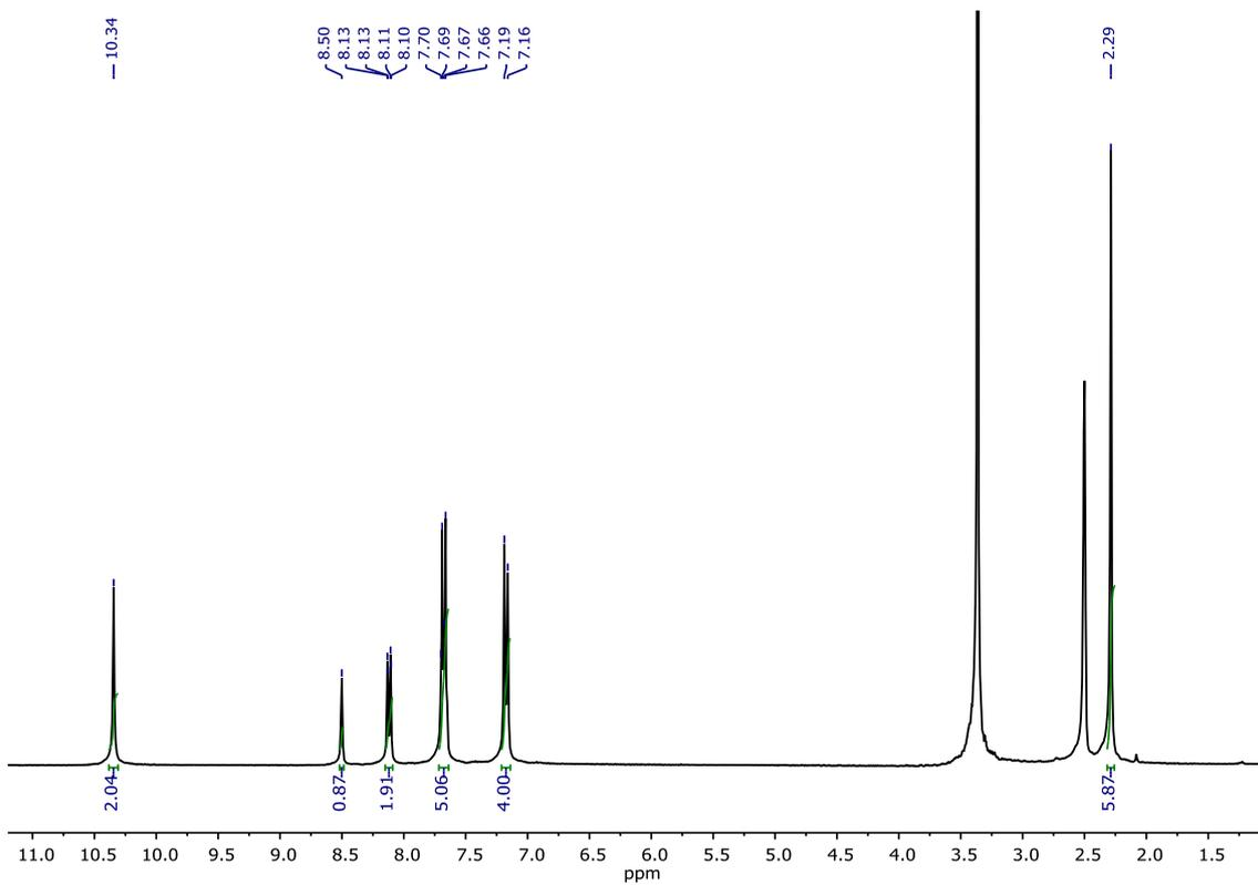
Figure S2.  $^1\text{H}$  NMR spectrum (300 MHz,  $\text{DMSO-}d_6$ ) for compound L1.
