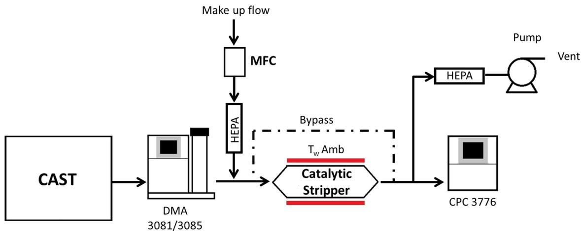
Figure S5. The experimental setup used to determine the particle losses of the CS at ambient T.
