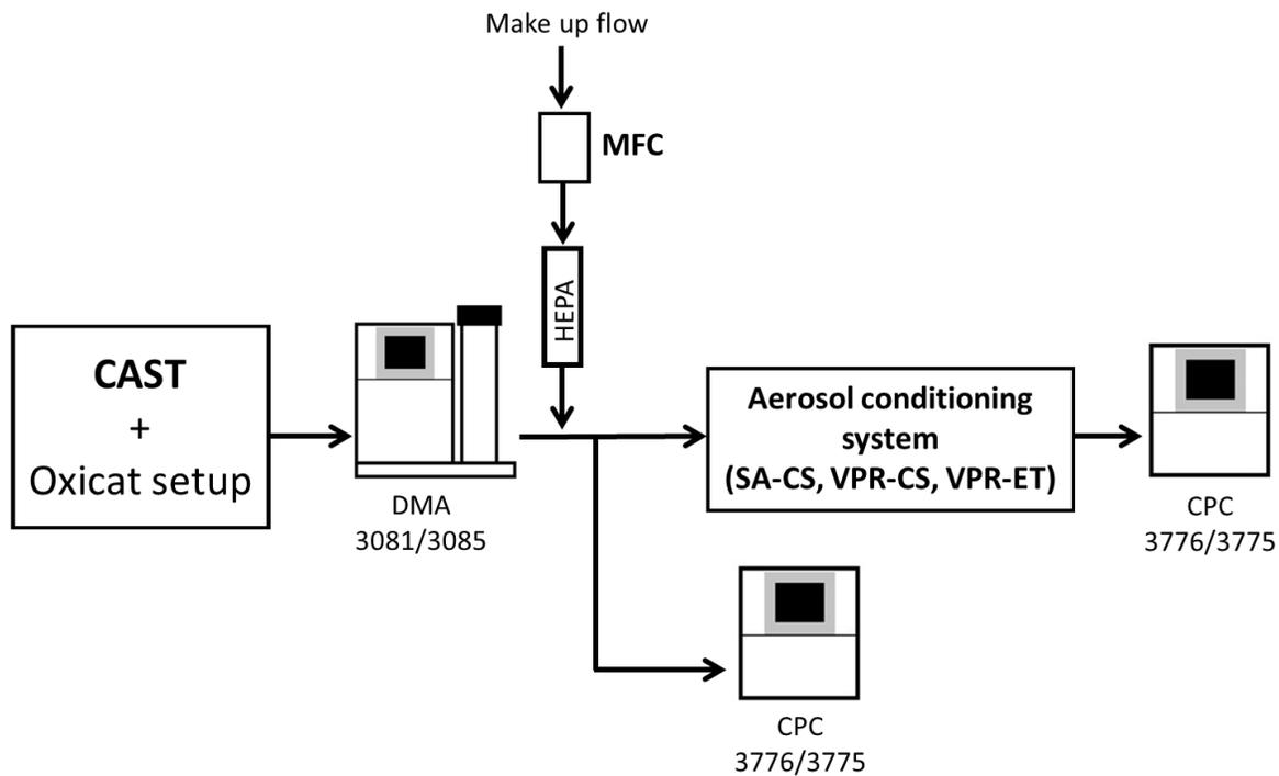
Figure S6. The experimental setup used to determine the particle losses of the SA-CS and the PCRF of the VPR-CS and the VPR-ET.
