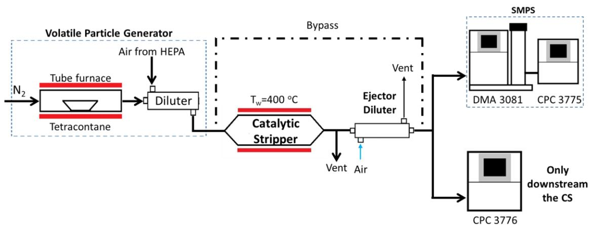
Figure S1. The experimental setup of tetracontane particle removal with the catalytic stripper as a stand-alone device.
