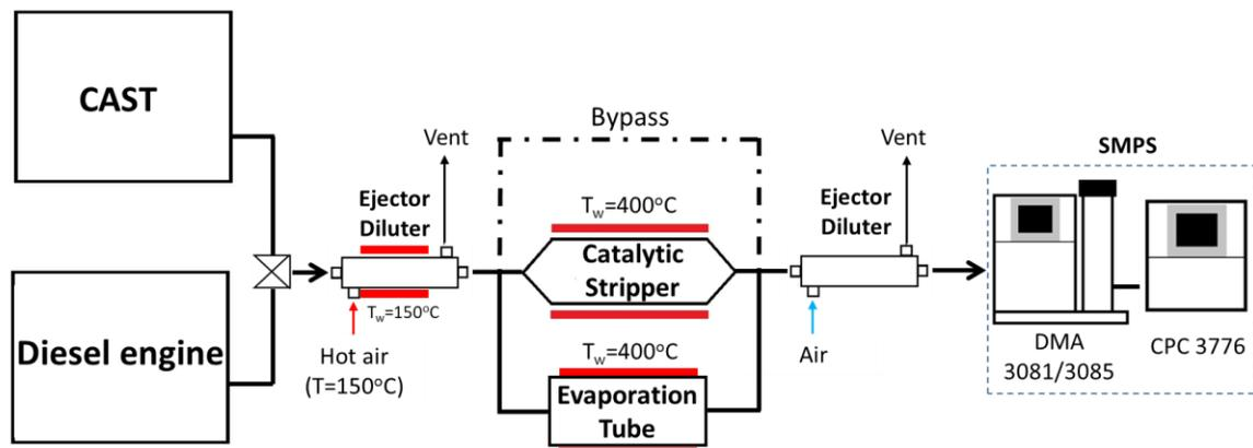
Figure S3. Experimental setup used for comparing the volatile particle removal efficiency (CAST generator) and the particle losses (Diesel engine) of two volatile particle removal (VPR) setups equipped either with a catalytic stripper (VPR-CS) or with an evaporation tube (VPR-ET).
