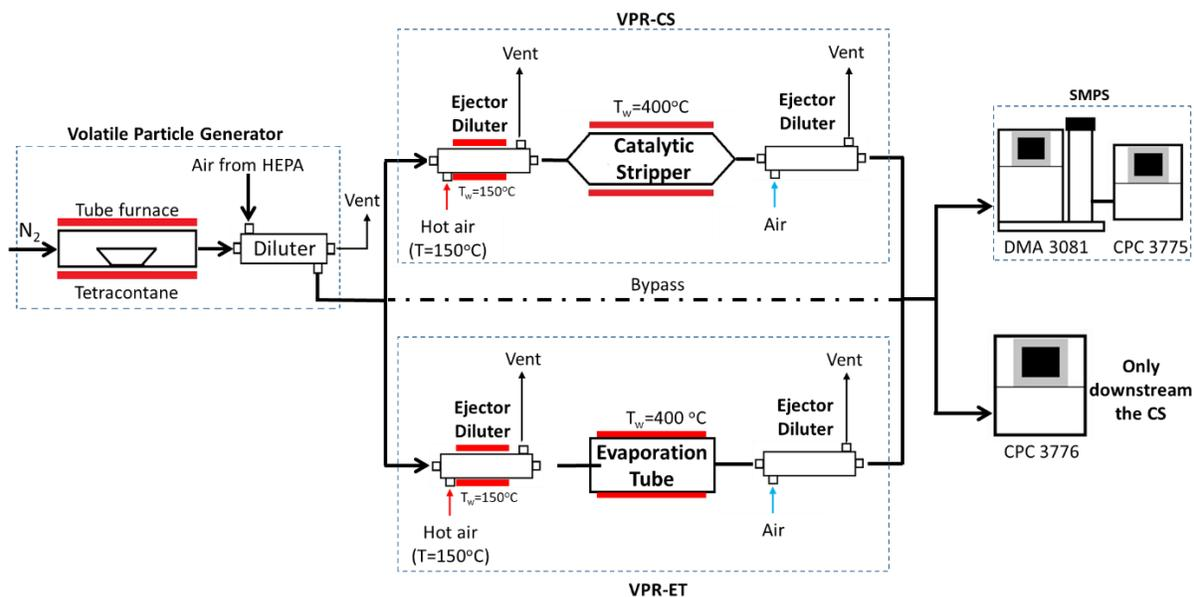
Figure S2. The experimental setup used to evaluate the C<sub>50</sub> removal efficiency of the VPR-CS and VPR-ET.
