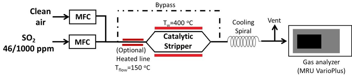
Figure S4. Experimental setup employed for the catalytic stripper's sulphur storage capacity study.
